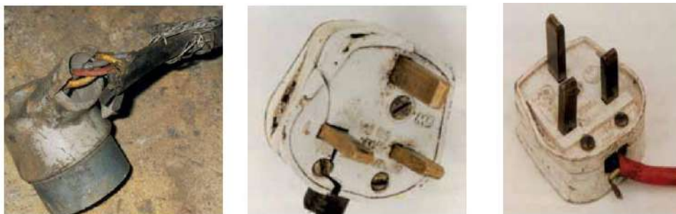
Figure 7.3: Electrical safety issues. Damaged cable grip (left), cracked casing (centre) and damaged cable sheath (right) [34]
